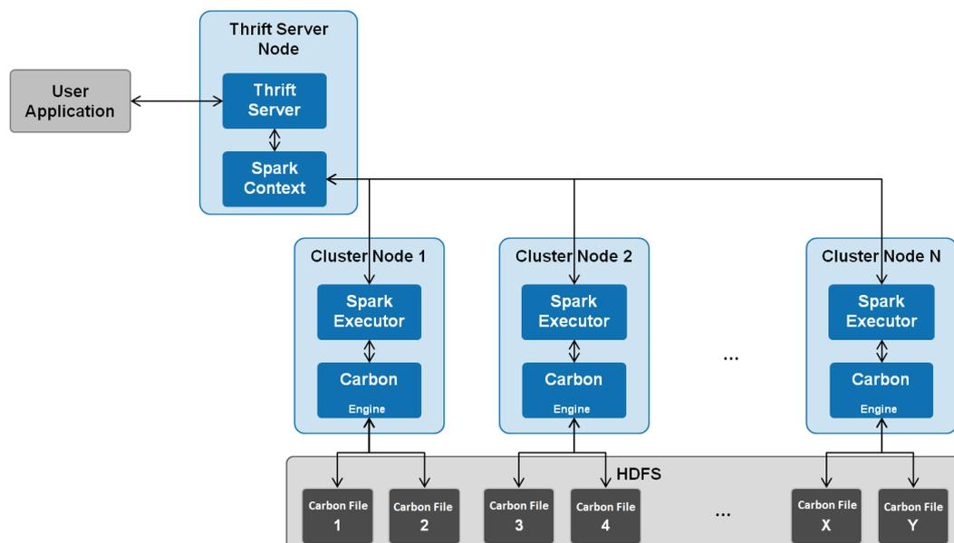
Data stored in CarbonData Table is divided into several CarbonData data files. Each time when data is queried, CarbonData Engine reads and filters data sets. CarbonData Engine runs as a part of the Spark Executor process and is responsible for handling a subset of data file blocks.
