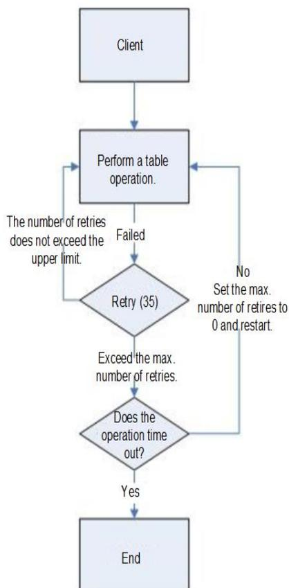
The process indicates that a suspension occurs if the preceding parameters are not configured based on site requirements. It is recommended that a proper timeout period be set based on scenarios. If the operation takes a long time, set a long timeout period. If the operation takes a short time, set a short timeout period. The number of retries can be set to **(hbase.client.retries.number)\*60\*1000(ms)**. The timeout period can be slightly greater than **hbase.client.operation.timeout**.
