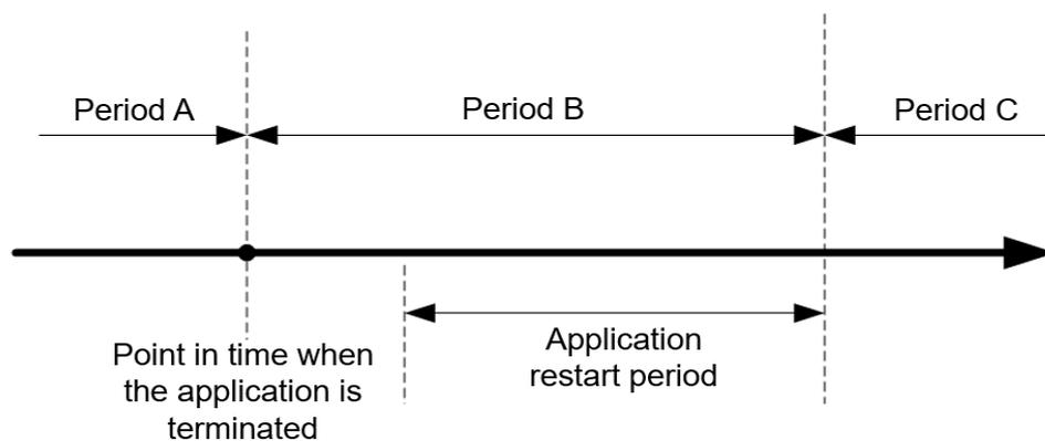
After this function is enabled, Spark preferentially schedules tasks in Period C. If there are multiple tasks in Period C, Spark schedules and executes the tasks in the sequence of task generation. Then Spark executes the tasks in Periods A and B. For data that enters Kafka in Period B, Spark generates tasks based on the end time
