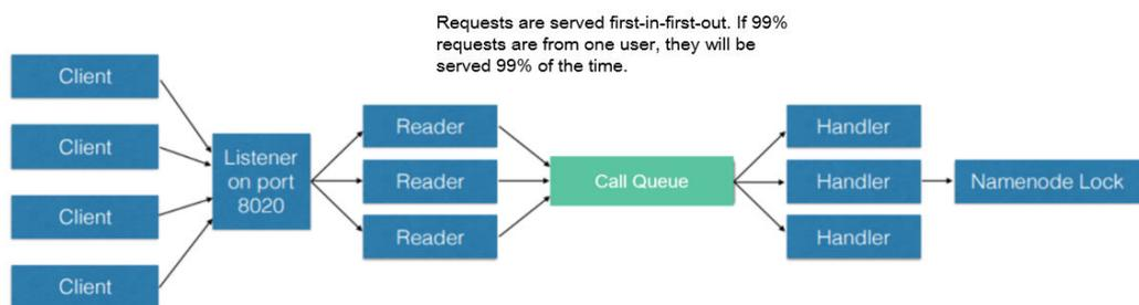
The unfair problem and delaying mentioned before can be improved by replacing the FIFO queue with a new type of queue called FairCallQueue. In this way, FAIR queues assign incoming RPC calls to multiple queues based on the scale of the caller's call. The scheduling module tracks the latest calls and assigns a higher priority to users with a smaller number of calls.
