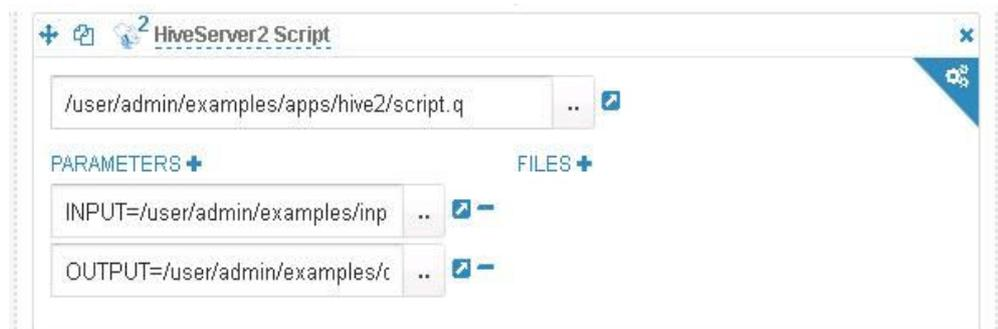
**Step 5** Click the configuration button
