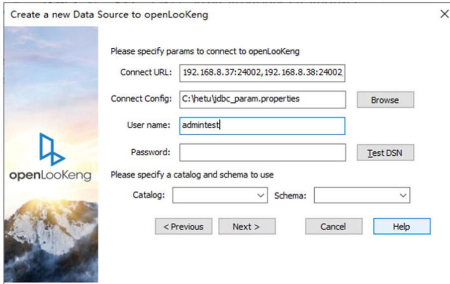
**Step 7** Click **Test DSN** to test the connection. If the connection is successful and both **Catalog** and **Schema** contain content, the connection is successful. Click **Next**.
