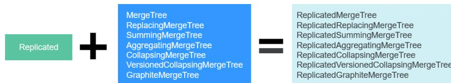
Replicated series engines use ZooKeeper to synchronize data. When a replicated table is created, all replicas of the same shard are synchronized based on the information registered with ZooKeeper.
