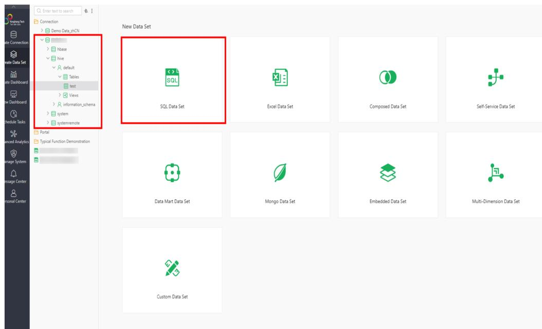
**Step 5** In the **Connection** area, select the new data set created in **Step 3**. All table information is displayed. Select a table, for example, **test**, and click **Refresh Data**. All table information is displayed in the **Data Details** area on the right.
