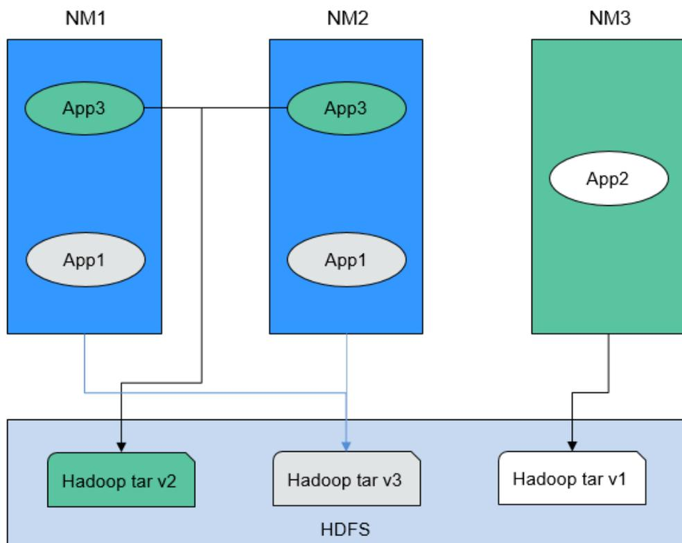
As shown in [Figure 14-1](#), the application can use Hadoop JARs in HDFS instead of the local version. Therefore, during the rolling upgrade, even if NodeManager has been upgraded, the application can still run Hadoop of the earlier version.
