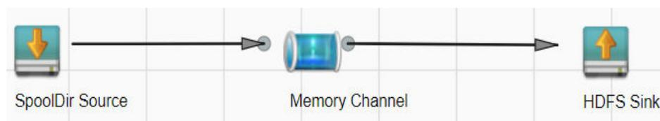
3. Double-click the source, channel, and sink. Set corresponding configuration parameters by referring to [Table 5-31](#) based on the actual environment.
