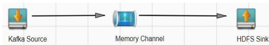
3. Double-click the source, channel, and sink. Set corresponding configuration parameters by seeing [Table 5-33](#) based on the actual environment.
