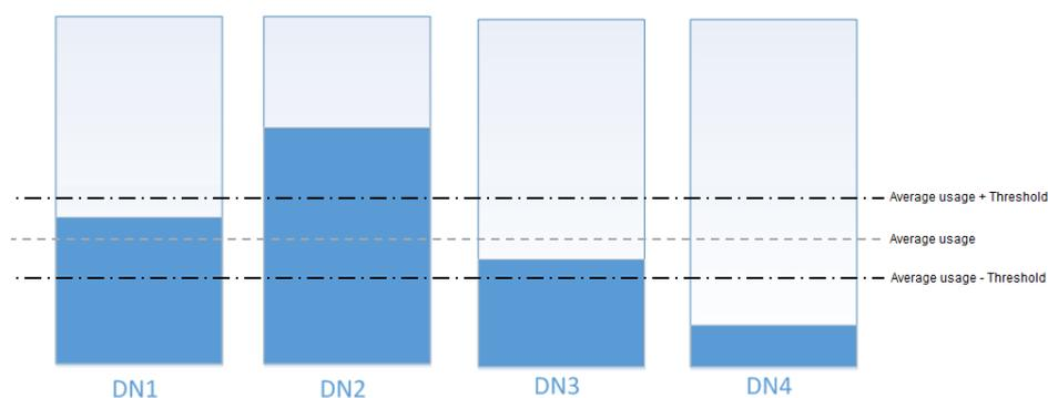
**Figure 7-2** DataNode disk usage after balancing
